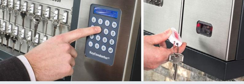
The next step is to decide if the system should be based on Barcode or on RFID Technology. If less than 150 keys or sets of keys are managed within your organisation, then often the Barcode option is chosen.
